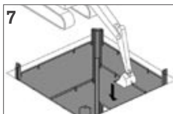
7 Excavator continues to dig and push the inside panels and corner posts...
