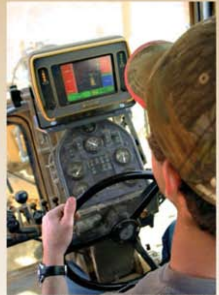
The control box mounted directly in front of the operator shows the precise position of the motor grader cutting edge, relative to finish grade, at all times.
